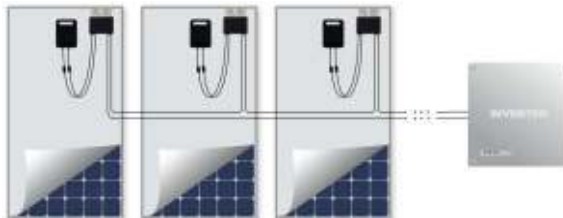
Figure 3: Power optimizers connected in series directly to a non-SolarEdge inverter
