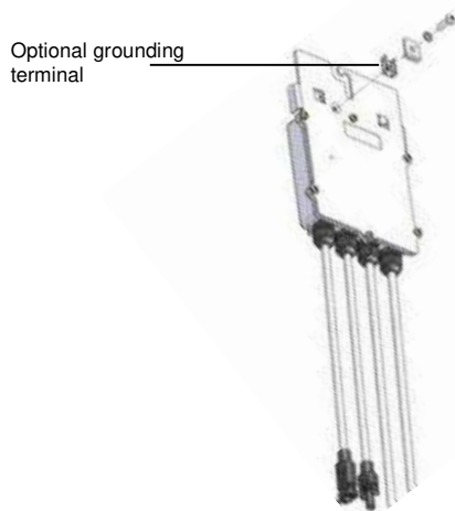
Figure 5: Power optimizer grounding terminal
