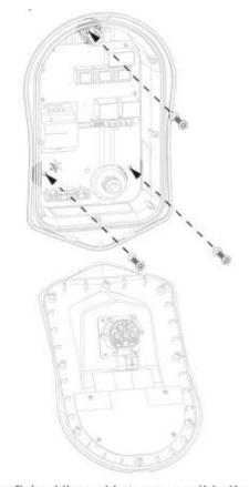
Using the fixing kit provided secure unit to the wall ensuring the grommets are used to maintain its IP integrity (Note: if using the rear cable entry remember to insert the mains cable before mounting to the wall!) 8
