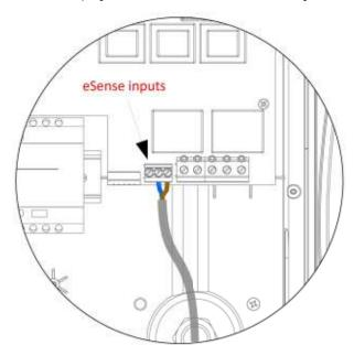
Connect the eSense cables using the opposite diagram
