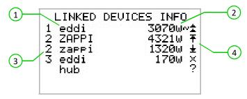
This screen lists all the linked devices 1 and the priority setting for each device 3 The current device is shown in CAPITAL letters. To the right of each device is the real-time output power level 2 The right side of the screen has symbols to show the status of each device 4 Refer to the table below for the meaning each symbol.
