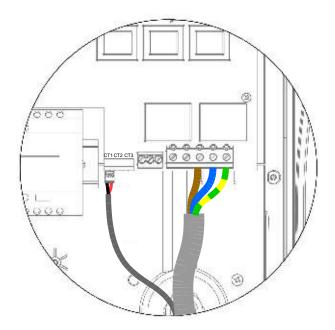
For single phase installations where 1 or 2 external / hardwiring an external CT please follow the above additional CT's are required, please follow the above diagram to connect the CT's using the extra 2 CT terminals in the same way if required.
