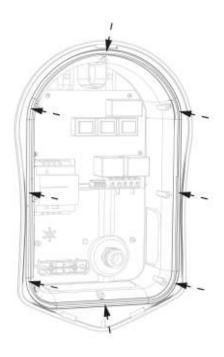
Ensure O-ring is present and sits neatly into its channel.
