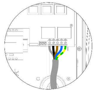
For 3 phase installations without the need for hardwiring an external CT please use the above diagram.
