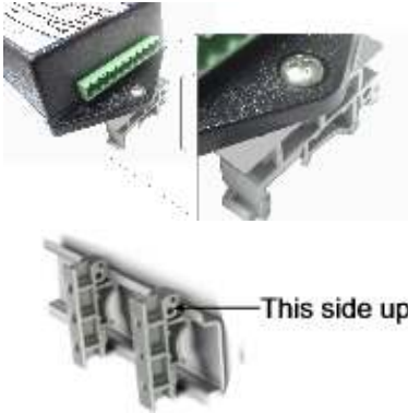
Figure 8: Mounting the meter on a DIN-rail
